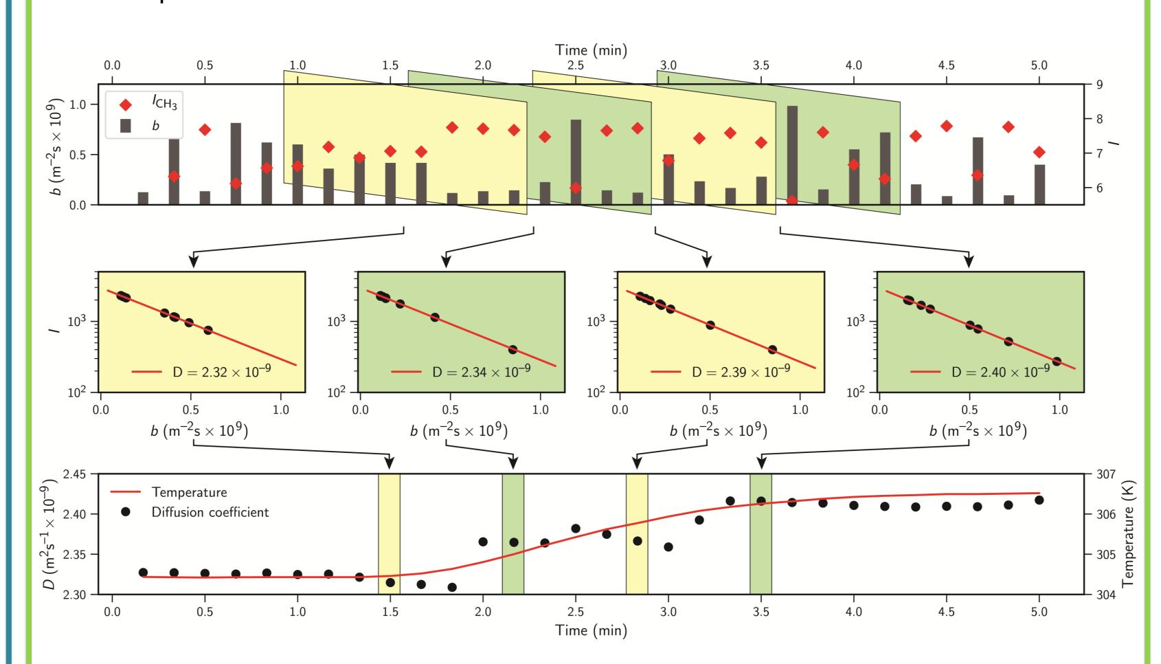
Diffusion NMR data with a time resolution of minutes obtained by moving-frame processing of a continuous dataset.
