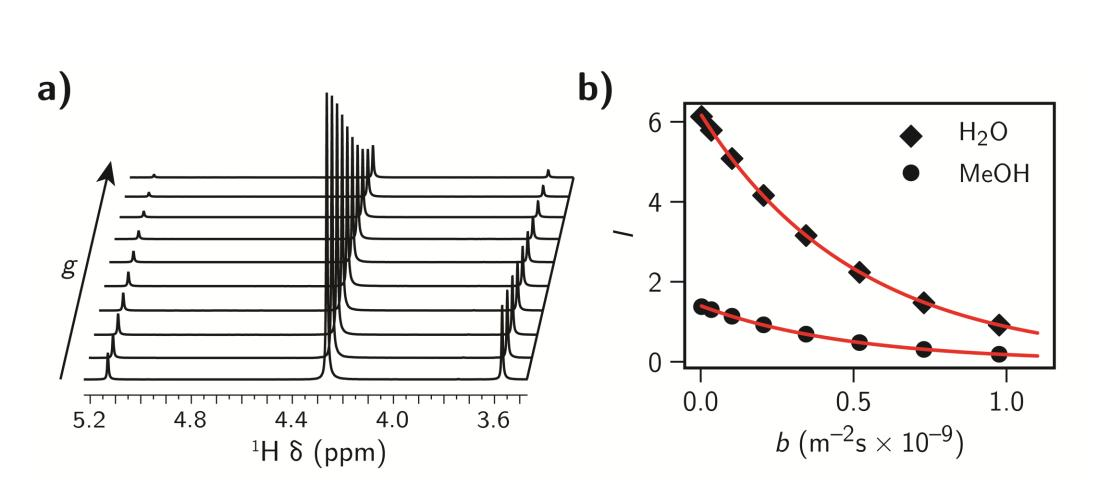
Diffusion coefficients can be measured by gradient NMR experiments, where signal intensities decrease as a function of gradient strength (above). Typical experiments performed on static samples can measure a diffusion coefficient within 5 – 20 minutes.
