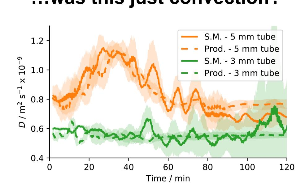
As a bulk phenomenon, convection (but not diffusion) is influenced by sample geometry. Repeating the reactions in narrow 3 mm NMR tubes eliminated (Pd-catalysed reaction, above) or sharply reduced (Grubbs RCM, below) the increase in measured *D.* "Enhanced diffusion" under these conditions appears to be an artefact.
