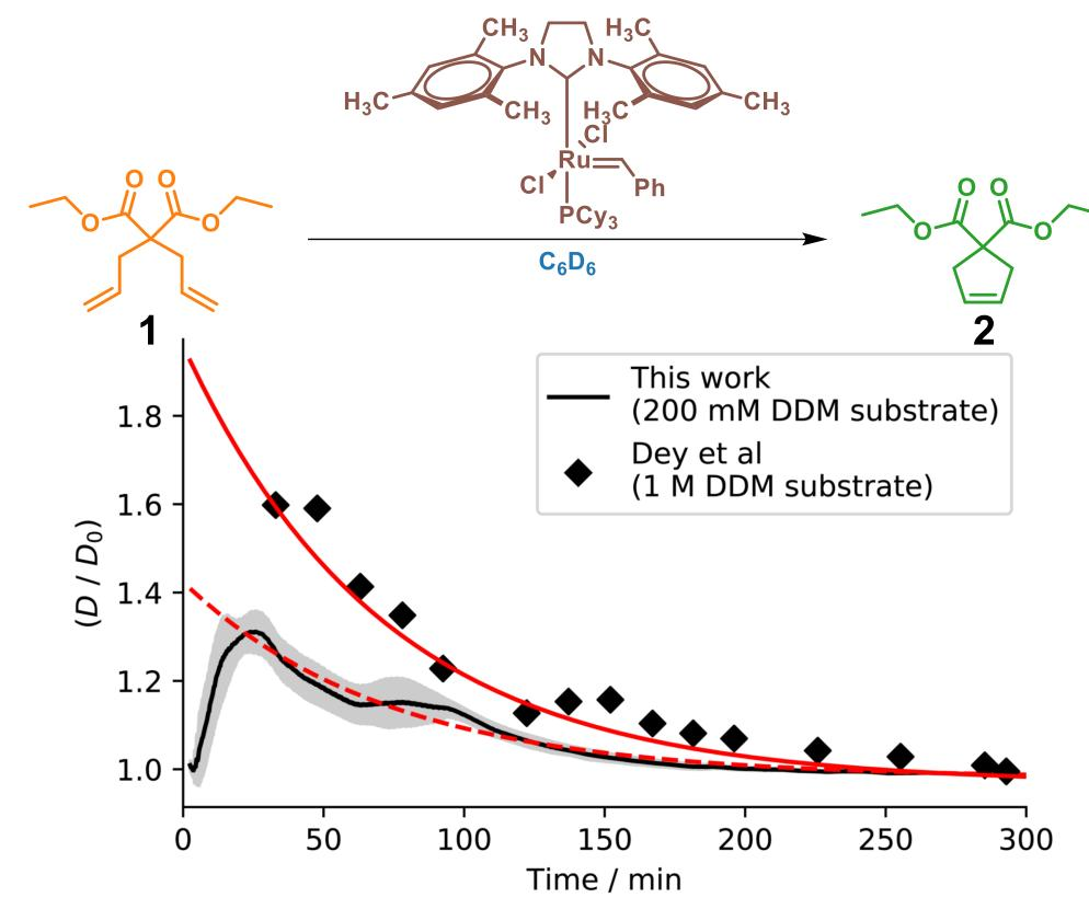
Enhanced diffusion of Grubbs' catalyst during metathesis.<sup>[2]</sup> Proposed models suggested a direct link between D and reaction rate (eg solid red line), but our time-resolved data<sup>[4]</sup> (black line) tells a different story.
